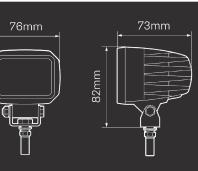
OVERALL DIMENSIONS 82 x 76 x 73mm CABLE LENGTH Approx. 370mm
